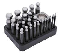
**Dapping Block and Punches:** This type of set is essential for the creation of spinner rings, as it's what's used to flare the ring so that the spinner bands cannot slip off. It's also used for making hollow round beads. This version is \$45 at Rio Grande (#112929), and another is \$38 at Otto Frei (#125.107). Really good sets will run into the hundreds of dollars, but for as often as you'll use this, you're better off investing that money elsewhere.
