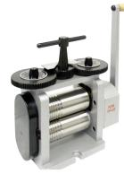
**Rolling Mill:** After you decide that shoes over \$20 are completely overrated, you'll be ready for a rolling mill. These are good for rolling patterns onto metal, reducing the thickness of metal, flattening solder, and fold forming. Expect to pay around \$600 or more for a good one.
